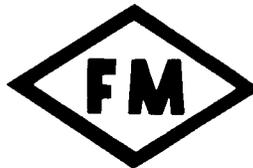
All FM. approved fire pumps will have the above identification mark on pump nameplate.
