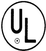
All UL. listed fire pumps will have the above identification mark on pump nameplate.
