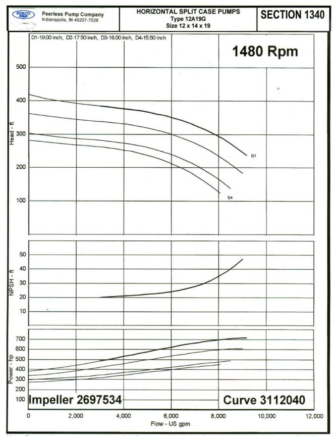
Note: Curves shown represents typical performance with Hydraulic Institute standard tolerance for 1.0 Specific Gravity fluids.
