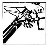
Batate Tool over Buckle, backing off with Tension Handle throughout entire course of bend. Failure to back off with Tension Handle throughout entire course of bend may result in breaking of Band. There is no loss of tension, as Band released is used up in the bend.
