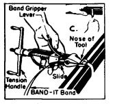
Draw Band snug (C). With thumb on Band Gripper Lever, apply tension with Tool.
