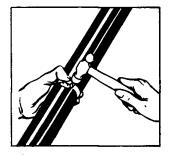
Clinch stub by hammering down Buckle ears, completing BAND-IT CLAMP.
