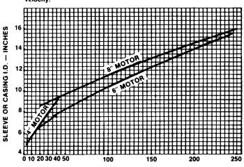
Double the flow for motors which require 1 ft/second minimum velocity.
