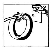
Bring end around object—preferably twice around and through Buckle. Bend end of Band under Buckle (B). For best results, apply Band twice around. Double banding develops almost four times the grip of single banding.
