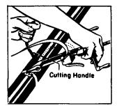
B Pull cutting handle to cut the Band.
