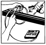
Band may be used from bulk roll as shown, or, for ease of application, cut off about 8' to 10' of Band; hook one end on Buckle (A) then bring the other around object to be banded and through Buckle.
