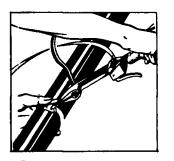
Remove Tool, holding stub of Band down with thumb.
