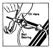
Apply proper amount of tension. (Band Gripper Lever locks itself under tension.)
