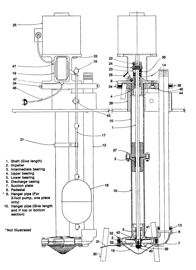
Figure 2. Type LG Vertical Sump Pump
