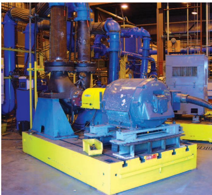
API between bearings double suction pump, Model 3620, on test on a closed loop system.
