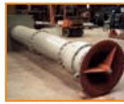
Fairbank Morse 24" Vertical Lift Pump
