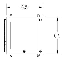
MTG FEET: 4 x 6.94" REAR MTG: 4.00 x 4.12
