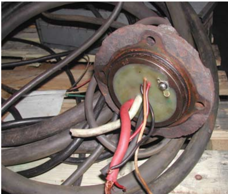
Figure 15. S.O.W. cords should be inspected for nicks and damage, otherwise the pumped liquids might wick down the cable to the motor interior.
