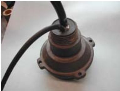
7. Pour the potting compound to the final level and make sure the leads are separated.
