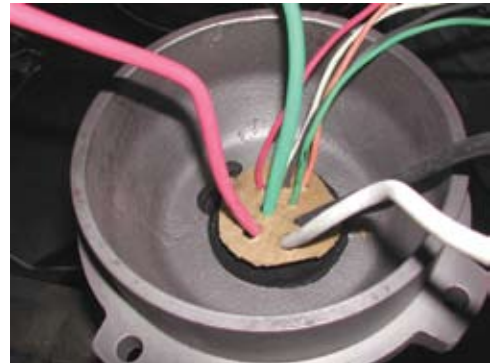
6. Fit the gasket to space the leads.
