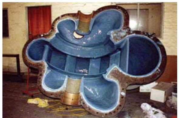
Figure 13. A variety of specialty ceramic coatings can be used to reduce the surface roughness and improve efficiency.
