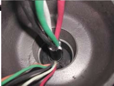
6. Fit the gasket to space the leads.
