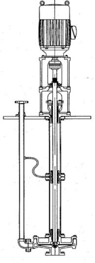
Taber Vertical Centrifugal Pumps 1000/8000 Series Chemical Process Sump Pump
