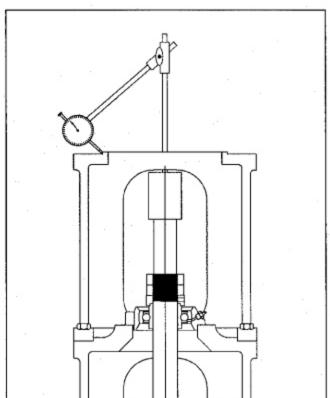
misalignment. The pump should not be operated with TIR > 0.010".
