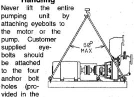
baseplate as shown). The total included hitch angle should not exceed 60°.
