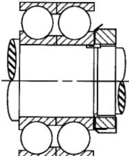
When bearings and shaft are cool, tighten the bearing locknut until lower bearing race is solid against the shaft shoulder. While the locknut must be tight, excessive tightening may damage the bearing race or the retaining shoulder on the shaft. Hand tightening with a spanner wrench is the best method available. Bend a locking tab of the lockwasher into a slot on the locknut with which it aligns. Completely cover the bearings to keep them clean.
