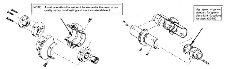
NOTE: Omega hubs are interchangeable with either standard or spacer flex elements: i.e., taper bushed hubs can be used with spacer elements and finished straight bore hubs can be used with standard elements.
