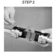
Place half of the elastomer element around hubs and secure with self-locking cap screws. The elastomer element will space the other hub. II is important to have cap screw properly tightened. See Table 1 below for recommended cap screw torgues and instructions. Now secure the other hub to the shaft.
