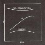
FIG. 6 Steam turbine horsepower rises with shaft speed.
