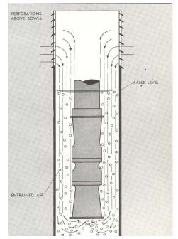
FIG. 2 FALSE DATA on water level occurs where there are perforations above the pump bowls.
