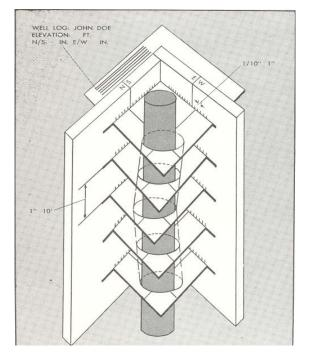
FIG. 1 THREE-DIMENSIONAL CONDITION of a well is best revealed by this slotted frame with adjustable cards instead of a graphical plot.
