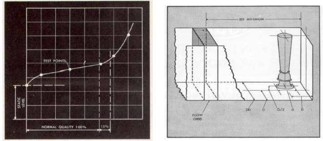
FIG. 3 PUMING SYSTEM PERFORMANCE is aided by a well production graph, and FIG. 4 Recommended from and dimensions for pump sump.
