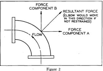
If the elbow is thought of as the eye of an impeller where the water turns in direction, it can be seen from Figure 3 that force component "A" will be cancelled out and the component "B" remains.
