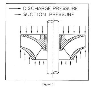
The forces causing thrust on a vertical turbine pump impeller can be pictured as in Figure 1.
