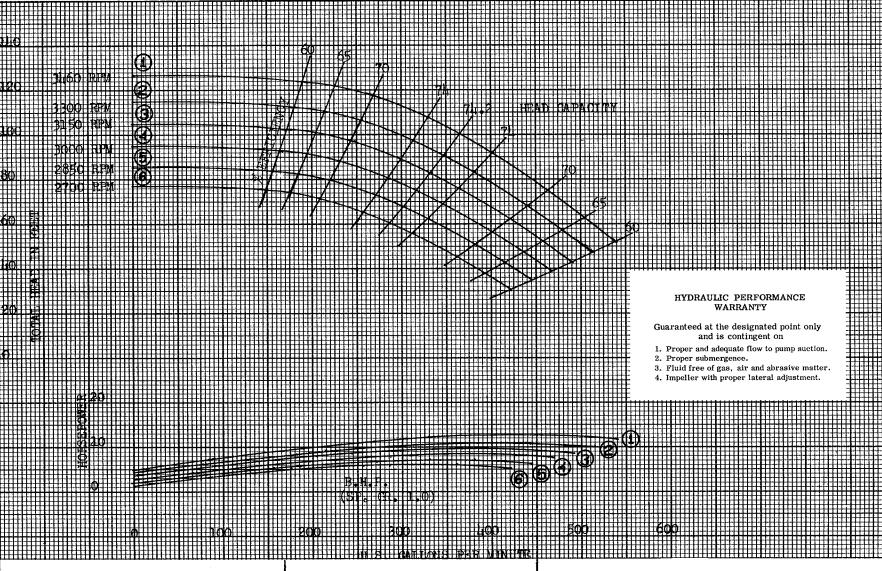
Impeller No 2620626 (brz or ci) Impeller Dia (full) 5-15/16" Bowl No 2620763 Reduce efficiency for special material bowls and impellers.
